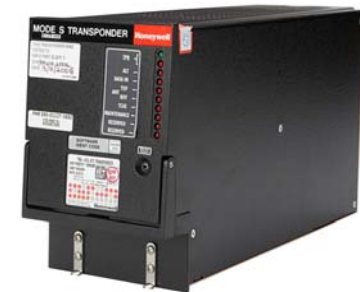
Honeywell TRA 67A Mode S ADS-B Out Transponder
